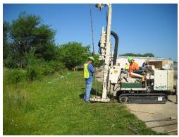
Figure 3: Direct Push Technology Drill Rig
