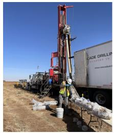
Figure 2: Sonic Drill Rig
